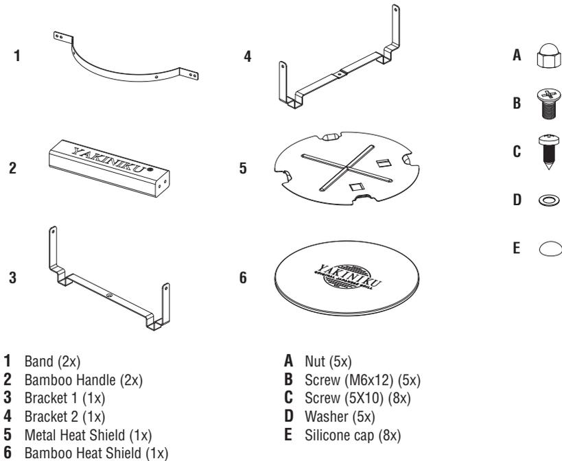
**STEP 1** - Manually attach Bracket 1 (3) to Bracket 2 (4) using an M6 screw (B), washer (D) and nut (A).
