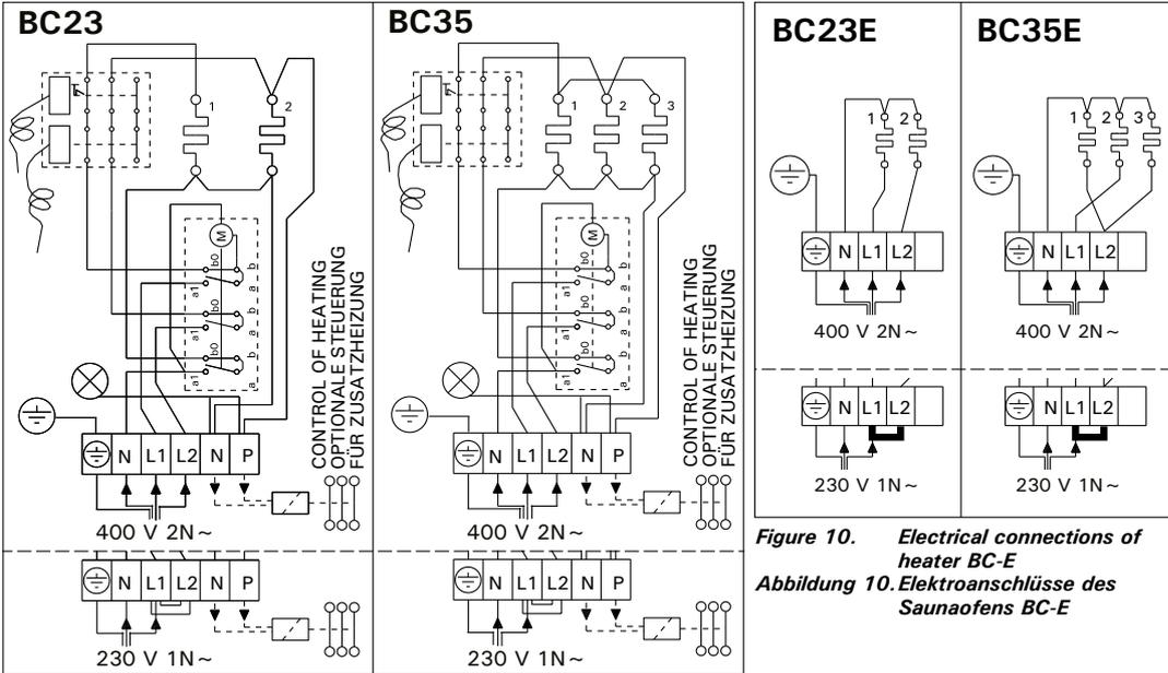
Figure 9. Electrical connections of heater BC
