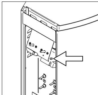
**Figure 8. Reset button for overheat protector**
