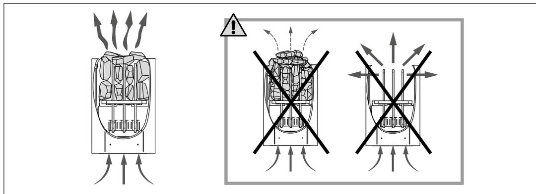
Figure 1. Piling of the sauna stones
