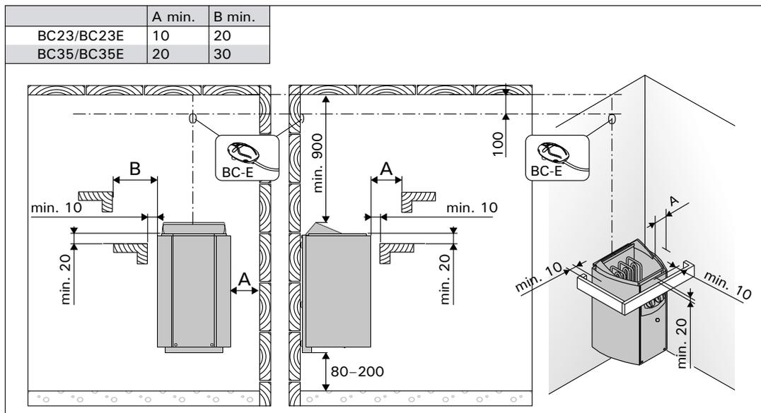
**Figure 6. Safety distances (all dimensions in millimeters)**
