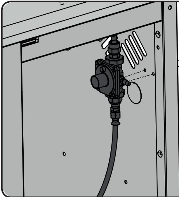
Fasten regulator to side panel using (2) M4 X 8 mm screws.
