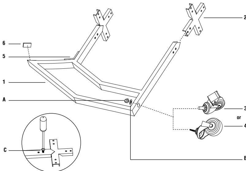
**STEP 1** - Attach 4x long gaskets/adhesive pads (5) and 4x short gaskets/adhesive pads (6) to the 4x upright leg sections (1) as shown. Make sure the long gasket (5) is attached to the inside of the angled leg section and the short gasket (6) is attached to the end of the upright leg section (1).
