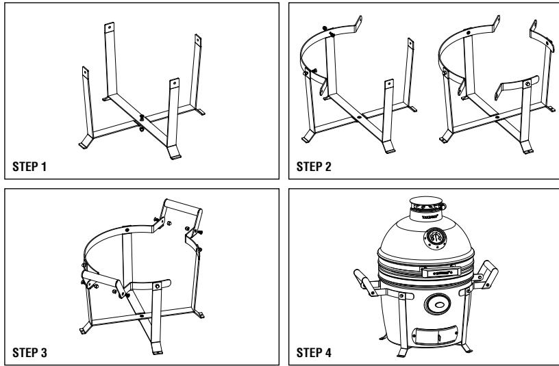
**STEP 1** - Insert the screw (B) through the hole of both Cart legs (1,2) and then tighten the cap nuts (A) by hand.
