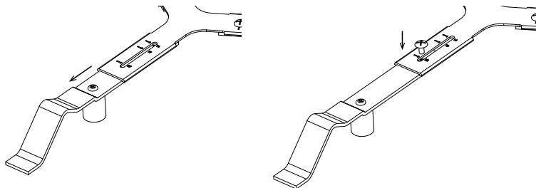
**STEP 1** - Adjust the table nest by extending the leg to the correct Kamado size, as indicated on the table nest.
