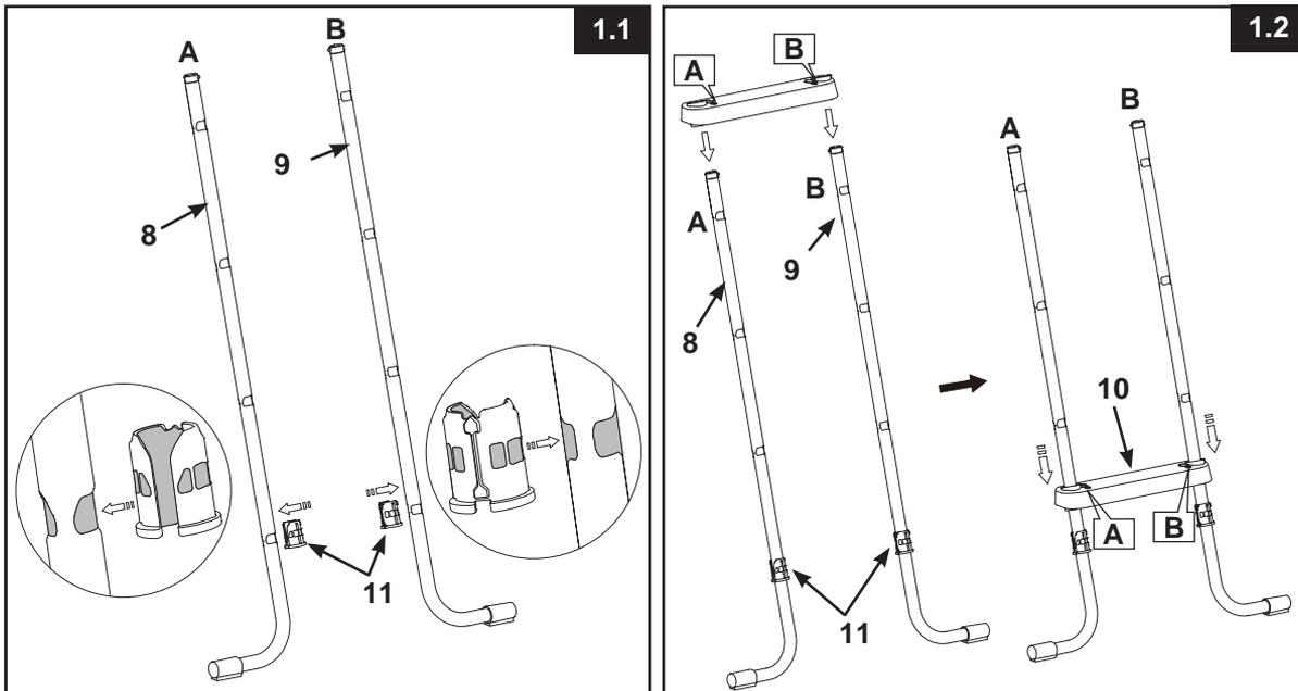
**IMPORTANT:** Ensure the J-shaped legs are pointing outwards before installing the steps.
