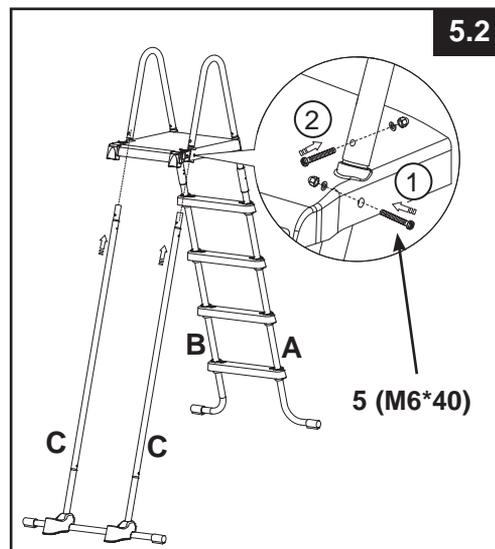
**IMPORTANT:** One side at a time. Do not attach the other side of the ladder until the U-shaped top rail is installed. Make sure all nuts and bolts are securely tightened. Do not fully tighten fasteners until last assembly operation.
