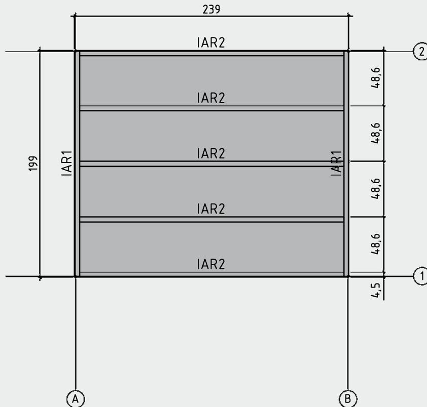
Floor boards - Fussbodenbretter - Plan pose plancher -
