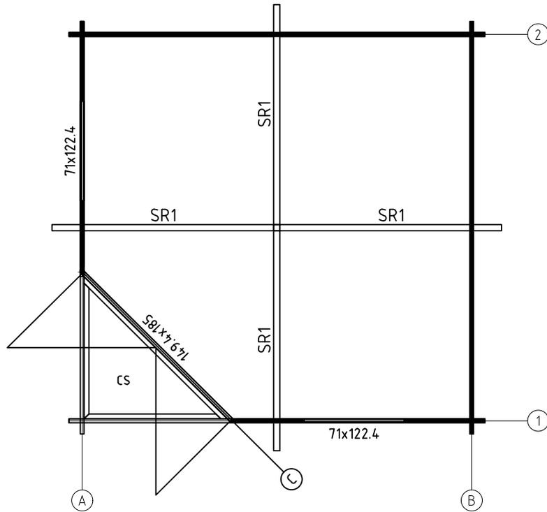
Diagonals must be equal A=B - Prüfung diagonale Austringug A=B -
