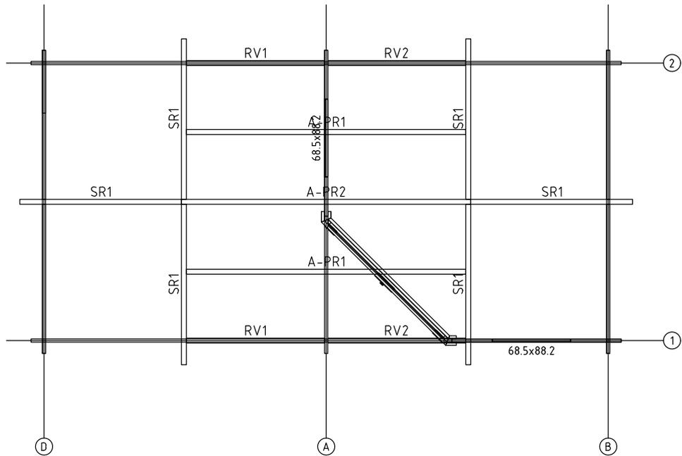
Diagonals must be equal - Prüfung diagonale
