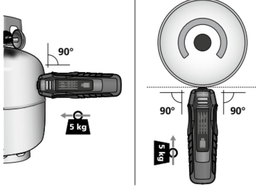
Place the measuring head vertically on the surface of the cylinder and press down applying approx. 5 kg of pressure.
