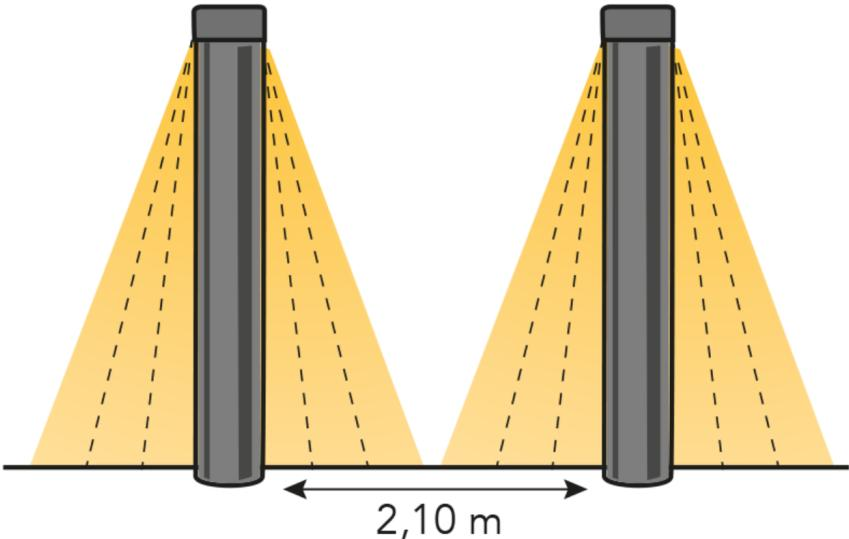
The diagram illustrates the lighting coverage of two identical cylindrical outdoor lights. Each light fixture is shown with a vertical cylinder and a yellow cone extending upwards from its top, representing the beam angle. The cones overlap slightly in the center. A horizontal double-headed arrow at the base of the cones indicates a distance of 2,10 m between the centers of the two lights.
